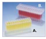
bottom and holds 5ml. The polypropylene unit measures 118 x 38 x 46mm high (4.6 x 1.5 x 1.8") and is autoclavable at 121°C (250°F). 3 per bag, reservoir cover and tray sold per each. PP A
